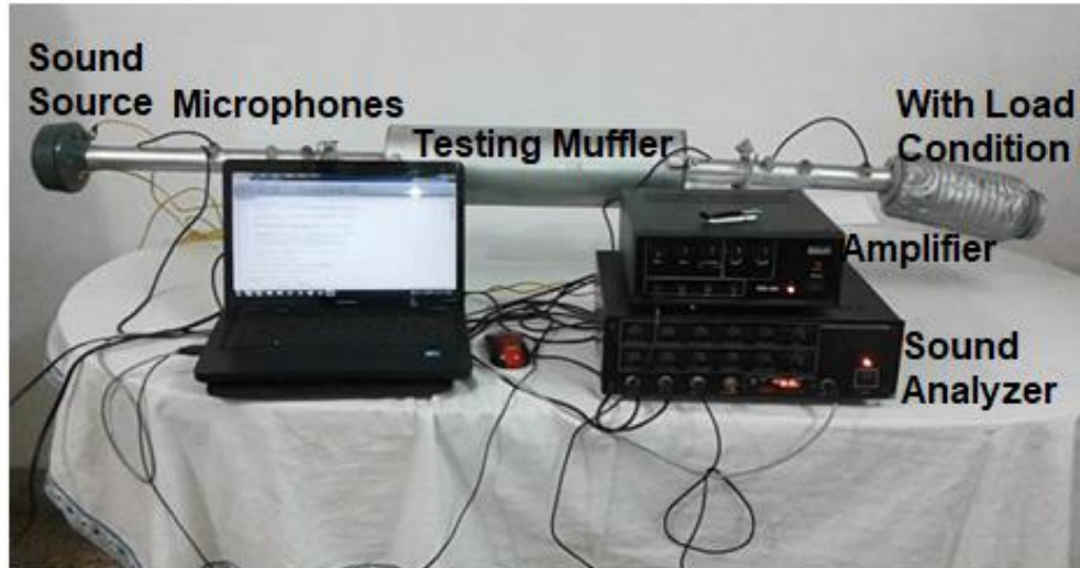
Figure 6: Experimental test rig setup for the evaluation of Transmission Loss for Hybrid Muffler
