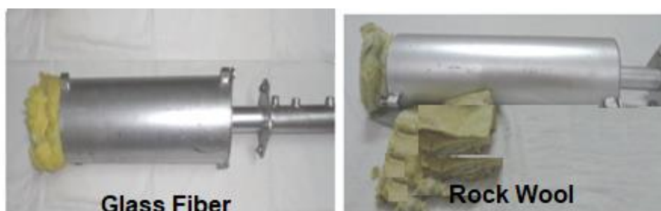
Figure 7: The unfilled muffler compartment comprises two main materials: (a) Glass wool and (b) Rock wool.
