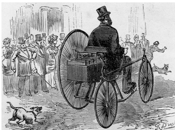
Figure-1: Gustave Truves's Tricycle (1881), World's First Electric Car
